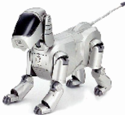
Figure 1. Aibo, Sony’s robo-dog with emotional behaviours, source: [www.world.sony.com/robot/get/m\\_instinct.html](http://www.world.sony.com/robot/get/m_instinct.html).
